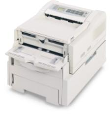
The network-ready OKIPAGE 12i/n (shown with standard 750-sheet paper capacity) ships with the OkiLAN<sup>®</sup> 310e+, a multi-protocol 10-Base T internal Ethernet<sup>®</sup> print server that delivers fast, simple and reliable network printing.
